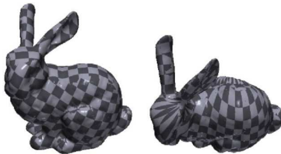
Figure 2: Texture mapping a checkerboard pattern onto a mesh model.
